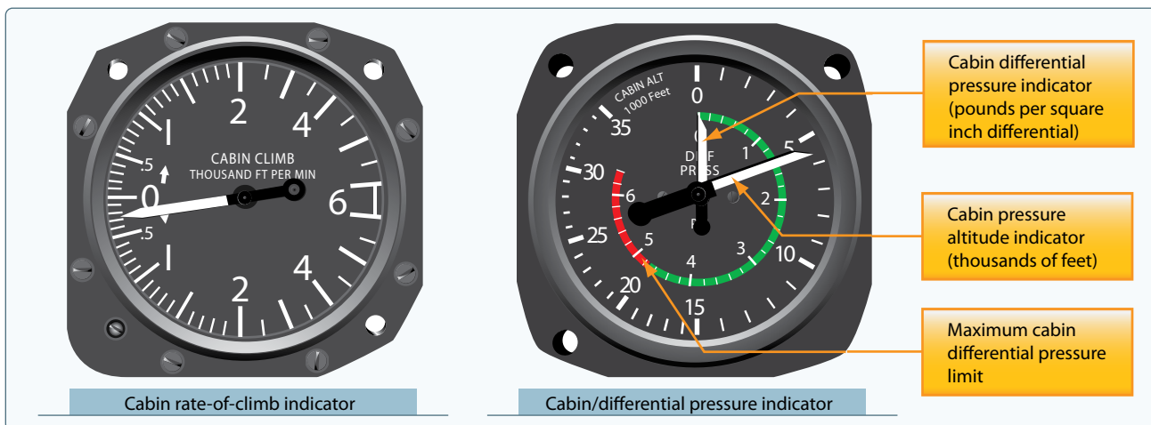
Figure 7-42. Cabin pressurization instruments.
