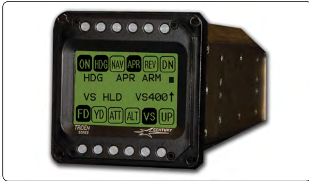
Figure 2-23. An example of an autopilot system.
