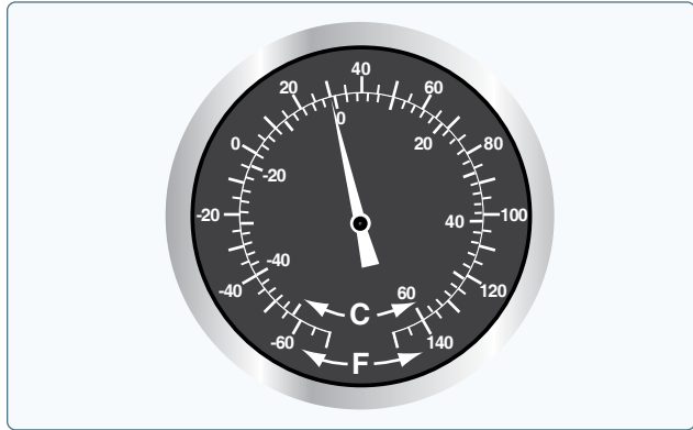
Figure 8-39. Outside air temperature (OAT) gauge.
