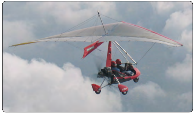
Figure 3-9. Weight-shift control aircraft use the shifting of weight for control.
