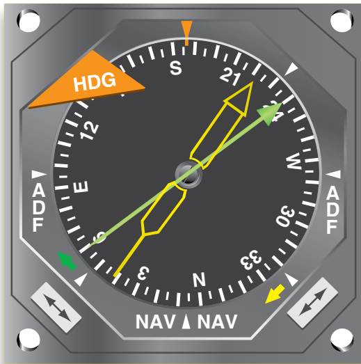
Figure 16-31. Radio magnetic indicator.
