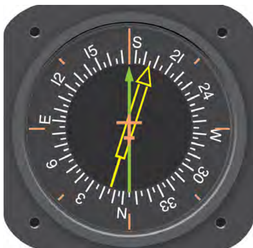
Figure 8-30. Driven by signals from a flux valve, the compass card in this RMI indicates the heading of the aircraft opposite the upper center index mark. The green pointer is driven by the ADF.
