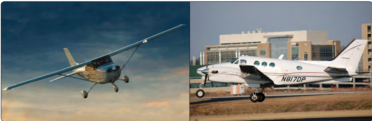
Figure 7-39. Fixed (left) and retractable (right) gear airplanes.
