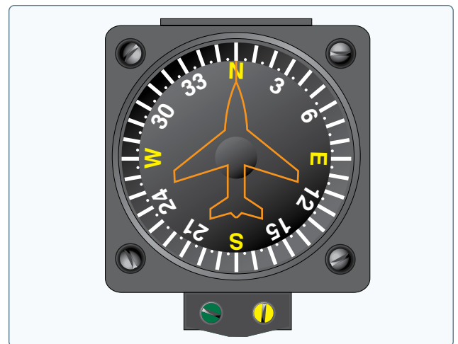
Figure 8-38. Vertical card magnetic compass.
