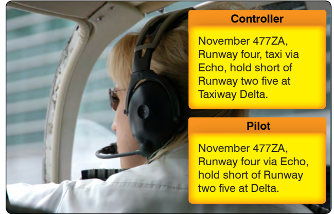
Figure 14-53. Example of taxi and “hold short” instructions from ATC to a pilot.
