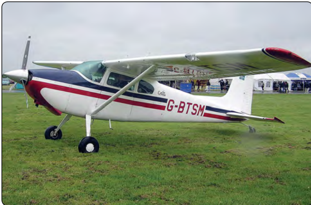
Figure 7-38. Tailwheel landing gear.
