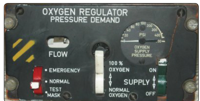
Figure 7-43. Oxygen system regulator.
